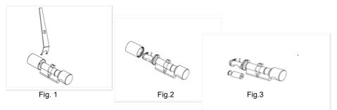
Use the special tool to loosen the locknut (Fig. 1) on the inner knob (long knob) approximately one rotation (only loosen slightly, do not unscrew completely). Carefully push the inner knob back and forth so that the sealing cone loosens and then unscrew the inner knob completely (Fig. 2).
