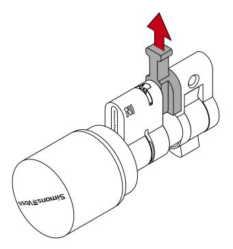
16. Push the halves together completely.
