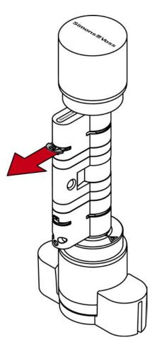
5. Disassemble the two cylinder halves.
