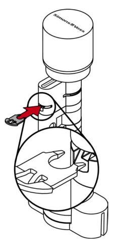
15. Insert the cylinder into the clamping block so that the profile cylinder and the thumb-turn lie flush in the recesses.
