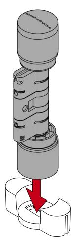
2. Attach the tip of the lifter into the clamp.
