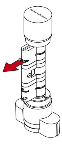
5. Disassemble the two cylinder halves.
