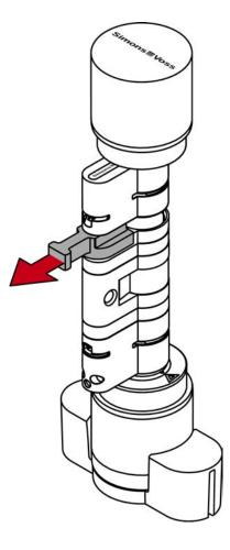
13. Push the halves together completely.
