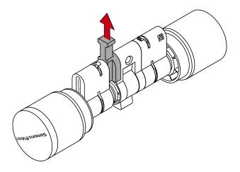
23. Push the halves together completely.
