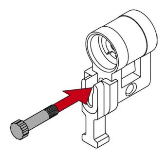
8. Place the prepared cylinder half in the thumb-turn assembly tool.
