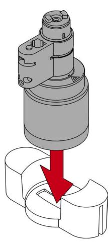
9. Place the half cylinder centre piece on the prepared cylinder half.
