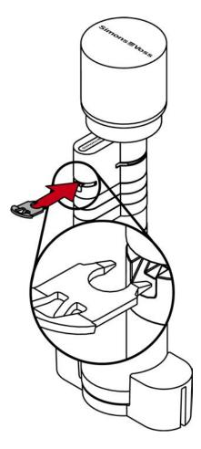
15. Insert the cylinder into the clamping block so that the profile cylinder and the thumb-turn lie flush in the recesses.
