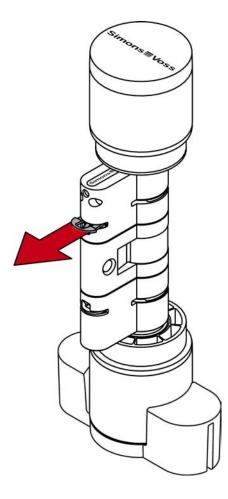
5. Disassemble the two cylinder halves.
