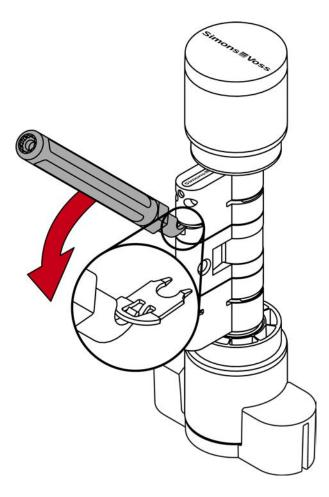
4. Pull the clamp completely out of the profile cylinder.
