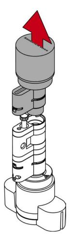
6. Use the extractor to unscrew the extension bolt.
