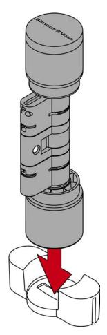
2. Hook the tip of the extractor into the clamp.
