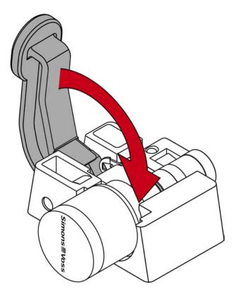
→ Half cylinder AX is fully assembled.
