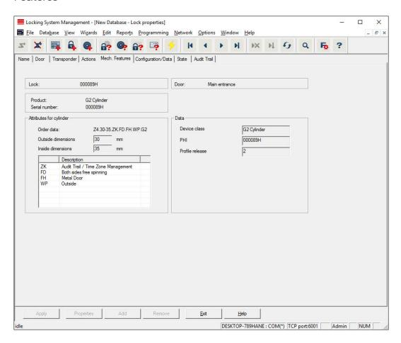
This tab shows the locking device's precise hardware options which are automatically entered during the initial programming.
