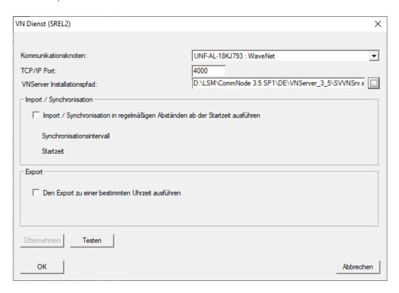
7. Optional: Go to the "Import/synchronisation" section and configure when the data from SmartRelay 2 G2 should be automatically imported back into LSM.
