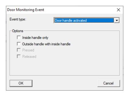
The following states can be detected. A check mark triggers the event as soon as the condition occurs:
