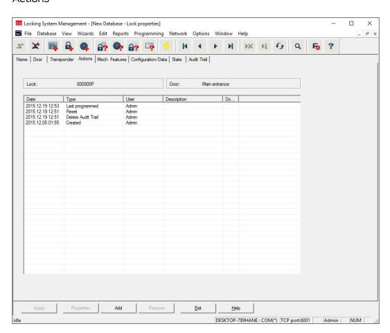
This table shows which actions (e.g. programming, authorization change, etc.) were carried out during locking. Different actions, such as "Last battery replacement", can also be added manually using the "Add" button.
