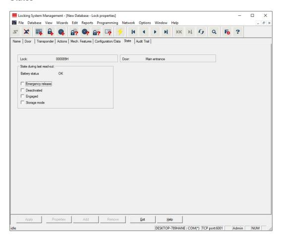
The last uploaded status of the locking device is displayed and is updated each time the locking device is read.
