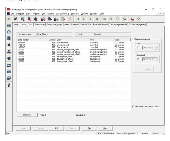
This tab gives you an overview of the locking devices used in the locking system. The devices are all displayed in detail in a table.
