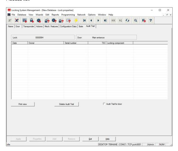
This tab can display the latest version of the access list. The locking device must support the "Access control" function, which must be enabled in the locking device properties.
