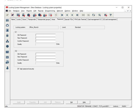
This is where you can change the locking system passwords used to change component programming.
