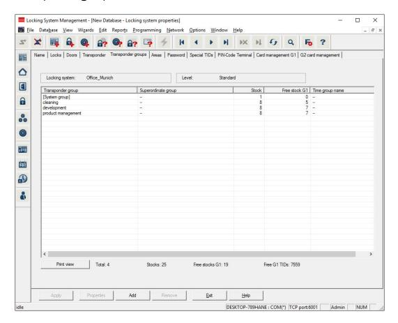
This tab gives you an overview of the transponder groups used in the locking system. The devices are all displayed in detail in a table.
