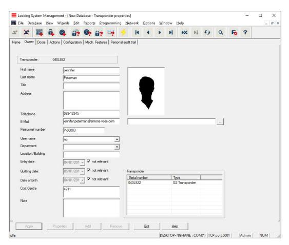
You can enter all information on the transponder's holder in the "Holder" tab. The "Transponder" table indicates how many transponders and which ones are assigned to the user. You can use the "..." to add a user photo. We recommend using JPEG images no larger than 500 kB.
