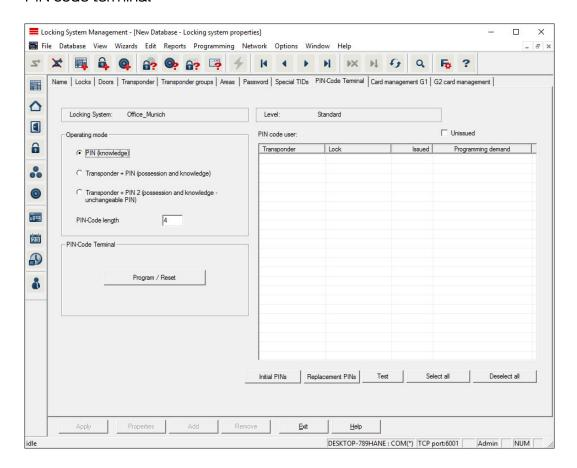
You can use this tab to add PIN code terminals and activate extended configurations.
