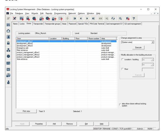
This tab displays the correlation between the doors contained in the locking system and their assigned areas. The devices are all displayed in detail in a table. It is possible to select one or more doors and assign them to a specific area, location or floor. Ensure that the areas, locations or floors have already been added.
