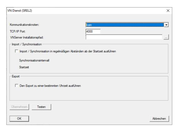
2. Select from the ▼ Communication nodes drop-down menu the communication node to which WaveNet with RouterNode 2 and SmartRelay 2 G2 is connected.
