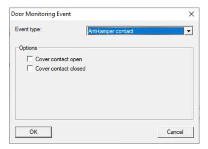
The following states can be detected. A check mark triggers the event as soon as the condition occurs:
