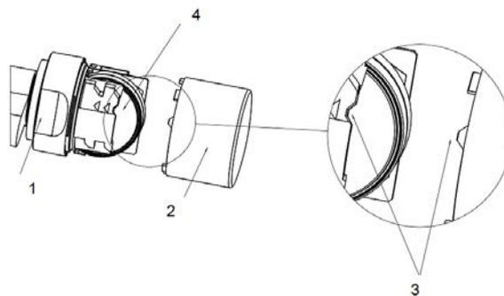
9. For MH cylinders only: Lock antenna back into place.
