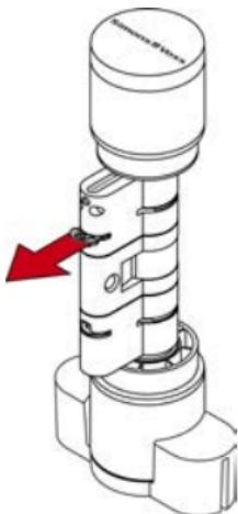
10. Disassemble the two cylinder halves.
