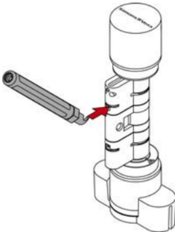
3. Lever the clamp out of the profile cylinder by moving the extractor to the centre of the cylinder.
