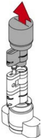
6. Unscrew the bolt with the extractor.
