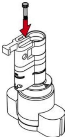
11. Reassemble the two cylinder halves.
