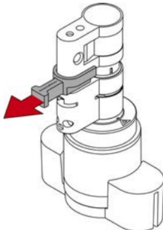
11. Push the cylinder parts together completely.
