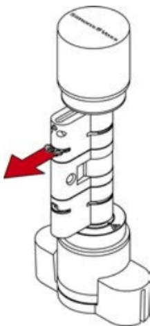
5. Disassemble the two cylinder halves.
