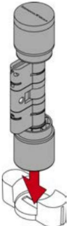
7. Hook the tip of the extractor into the clamp.
