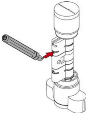
8. Lever the clamp out of the profile cylinder by moving the extractor to the centre of the cylinder.
