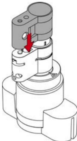
12. Refit the clip into the slot of the profile cylinder with the lug facing the fastening screw.
