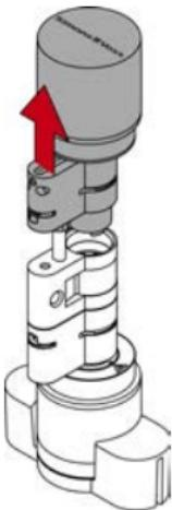
↳ First cylinder half prepared with centre piece and tappet piece.
