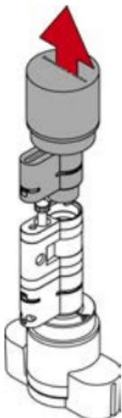
6. Use the extractor to unscrew the extension bolt.
