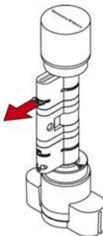
5. Disassemble the two cylinder halves.
