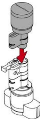
12. Refit the clip into the slot of the profile cylinder with the lug facing the fastening screw.
