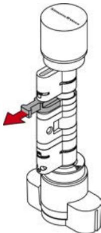
13. Push the halves together completely.
