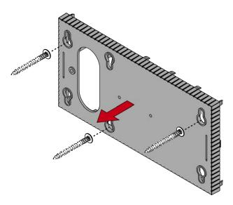
6. Slide the base plate so that the screw heads slide along the grooves.
