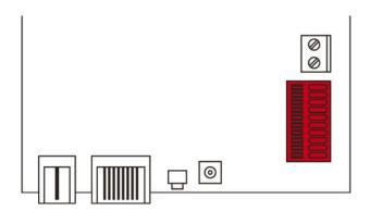
The IO connector enables you to communicate with external devices. Use a screwdriver to push the spring-loaded terminal downwards to connect or disconnect cables. Details and application examples for wiring the IO-Connector can be found in the RouterNode-2 manual.
