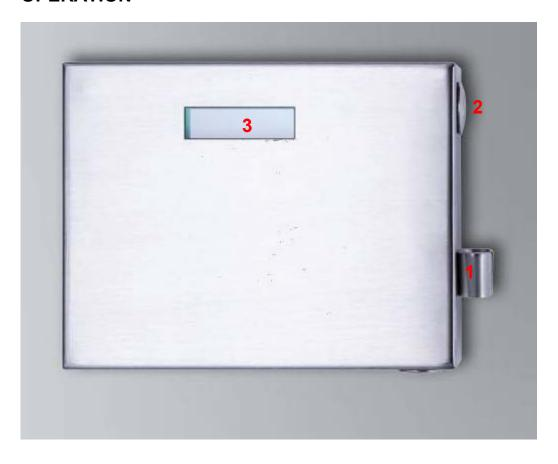
To ensure that the transponder is programmed correctly without any errors, you must place the transponder in the transponder bracket (1) and not hold it in your hand or place it on top of the housing. The bracket holds the transponder in a position where the range and alignment are optimally matched. The transponder bracket (1) is attached to the right-hand side of the housing.
